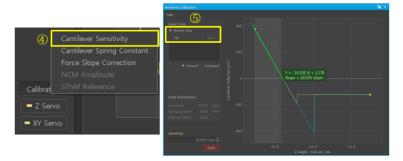
Figure 8-4-18. Sensitivity Calibration window
