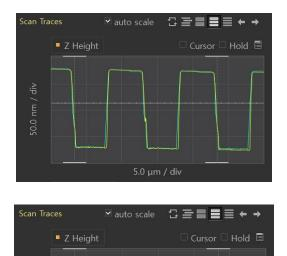
Figure 5-9. Proper Gain (top); Noise from Excessive Gain (bottom)
