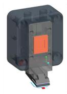
The NX-Hivac's Z scanner is separated from the X-Y scanner. This independenc e provides the user with several operational advantages.
