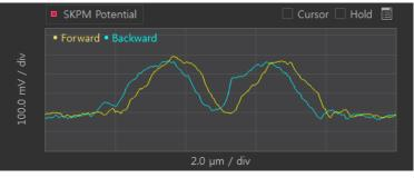
Figure 14-40-a displays a noisy line profile resulting from a large Tip bias servo gain value and Figure 14-40-c displays a blurry line profile resulting from a small Tip bias servo gain value. Adjust the Tip bias servo gain value to minimize line profile noise and synchronize forward/backward lines.
