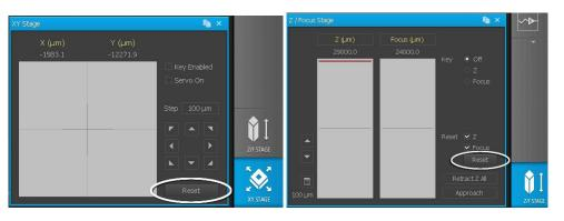
Figure 3-13. Reset the motorized Stages
