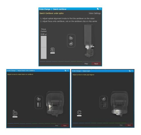
Figure 4-1-3. Searching Cantilever, Beam alignment and PSPD adjustment
