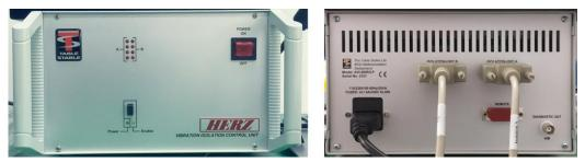
Figure 2-16. AVIS Controller (left: front, right: rear)
