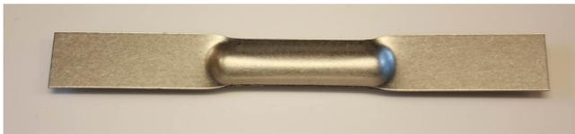
**Titanium** is very difficult to thermally evaporate because Ti will melt (1660 °C) at the same time that it reaches a temperature high enough to yield reasonable deposition rates. Molten Ti will react with most materials as it is a very corrosive material. Therefore the boats can be used only for one evaporation in most cases.
