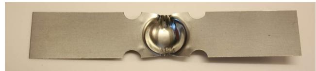
**Platinum** is a very hard evaporating material but it is not reactive with the boat source materials. Uses always evaporation source 4 for Pt evaporation. Recommended boat for Platinum in PVD75 is:
