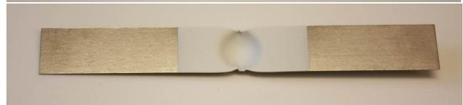
**Chromium** evaporation is more of a conceptual problem than a real problem. Chromium full sublimates and will not melt when thermally evaporated. It comes in irregularly shaped pieces. The Cr pieces do not react with the boat material and the boat can be reused many times. Use source 4.
