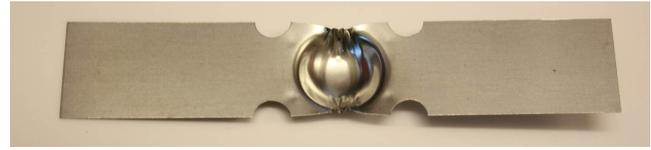
**Gold, Silver, Copper** are very gentle materials, they evaporate in moderate temperatures and relatively low powers. The boat can be reused many times.
