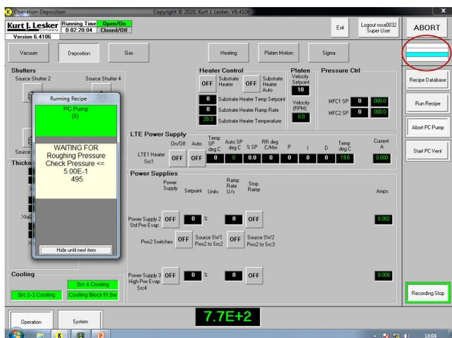
In the co-deposition Example, the step that does not work for mapping Output #1 is skipped. You will need to leave this step skipped and set it manually before running the recipe as described below.
