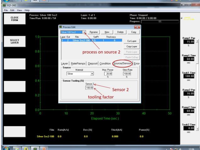
Another way to check and replace the tooling factor is: **Edit** ⇒ **Films** ⇒ **Source/Sensor** then select the correct process.
