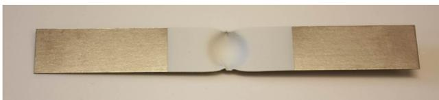
**Palladium** is similar to nickel in that when it is in liquid form (melts at 1554 °C) it is extremely reactive with the boat source materials and will destroy an Al<sub>2</sub>O<sub>3</sub> coated boat as soon as the Pd melts into a liquid. The Pd does attack and usually breaks the Al<sub>2</sub>O<sub>3</sub> coated boat when a second run is attempted. Recommended boats for Palladium in PVD75 are:
