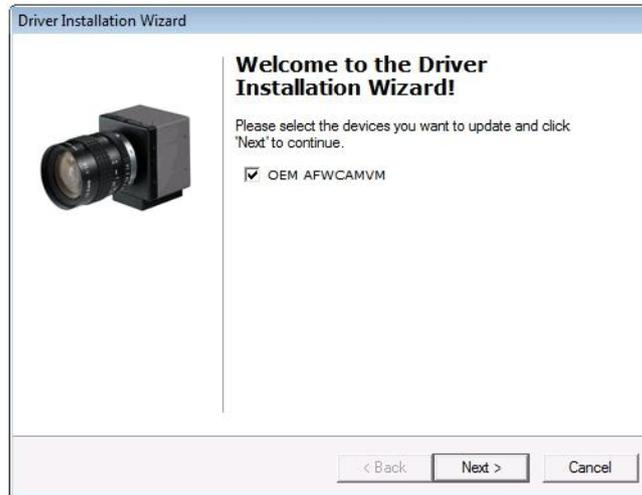
If the ImagingSource camera driver was selected a Driver Installation Wizard will start up. All the connected & detected ImagingSource cameras will be listed. Usually only the Theta ImagingSource camera will be listed (but named as shown above). Ensure that the tickbox is checked and click *Next*.
