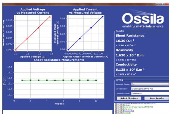
6. Measure at different points on the sample for better accuracy. The precision of the measurement with this system can vary between 0.05% up to 5% depending on the sample and system setting parameters. Precision is the maximum deviation between identical measurements (useful for comparative measurements).
