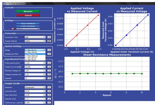
4. Click the Measure button. The system will then try to apply the set target current between the outer two probes. Once this has been achieved, the voltage will be measured between the inner two probes and the sheet resistance calculated from these values. Once the measurement has finished, the average sheet resistance will be displayed in the results box on the right side of the window.
