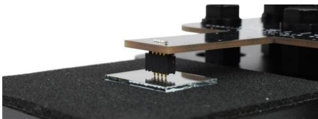
2. Use the micrometer to raise the stage until the probes are in good contact with the sample. As the probes are spring-loaded, they will compress as the sample is raised into them - creating a constant contact force. If the sample is not centered, lower the stage until the probes are not in contact before repositioning it to prevent damaging the sample.
