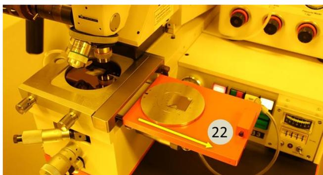
19. When the desired exposure time is over: Pull separation lever all the way forward you. The lamp shutter will close.
