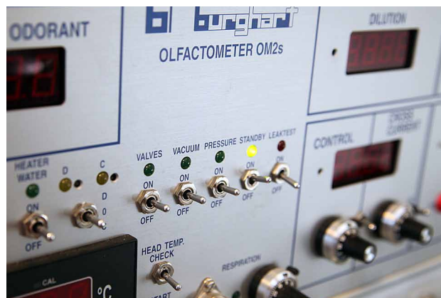
The olfactometer used during the fMRI-experiments to expose the participants to different kinds of odours.
